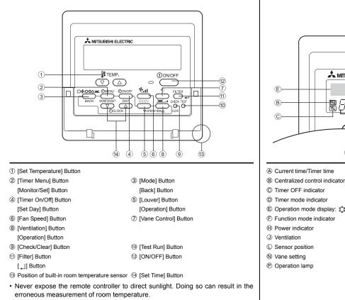
· Never place any obstacle around the lower right-hand section of the remote controller. Doing so can result in the erroneous measurement of room temperature.
