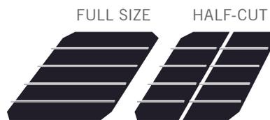
Innovative half-cut cells reduce the electrical current carried by each busbar by half, decreasing electrical resistance and increasing overall efficiency by 2.5%.
