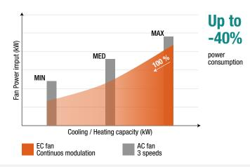
The inverter technology allows continuous, stepless airflow and capacity modulation so that the unit can easily follow any variation in the thermal load.
