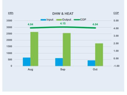
\*1 Based on the unit's August 2021-October 2021 electrical consumption (1698 kWh) and heat delivery through heating and hot water (6925 kWh).
