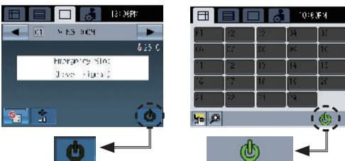
If the external input interface receives an emergency stop signal, all indoor units, LOSSNAY, and Air To Water (PWFY) units that are controlled by the AT-50B will stop. The AT-50B controller, low-level system controllers, or local remote controllers will not respond until the emergency stop signal input is removed. When the emergency stop signal is removed, the operation status before the signal was received will be restored.
