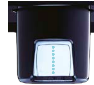
8 Sensors measure while moving left to right
