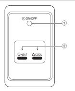
(1) ON/OFF lamp (lit when unit is operating; unlit when unit is not operating)
