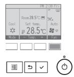
Press the [F4] button to go through the fan speeds in the following order.
