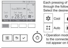
Each pressing of the [F1] button cycles through the following operation modes. Select the desired operation mode.
