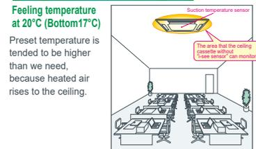
With i-see sensor\*Auto fan speed: preset temperature at 20°C
