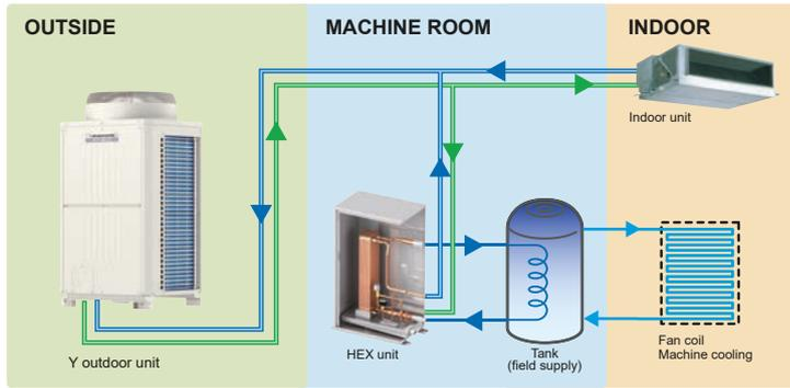
The HEX unit is connected to the Y series outdoor unit with refrigerant pipes, and to the water tank with water pipes. The HEX unit is not equipped with a compressor.
