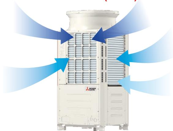
Efficient air suction is achieved by placing the heat exchangers on the upper part. The multiplier effect created by increasing the number of suction surfaces from three surfaces to four surfaces greatly improves the operation efficiency.
