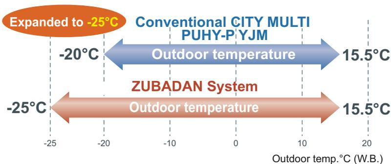
From a previous LOWEST operating ambient temperature of -20°C, the ZUBADAN System pushes the boundaries of technology to give heating in ambient temperatures as low as -25°C.
