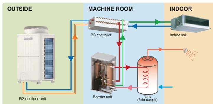
The Booster unit is connected to a BC controller with refrigerant pipes, and to the water tank with water pipes. The waste heat from cooling operation is utilised for heating operation to provide hot water.
