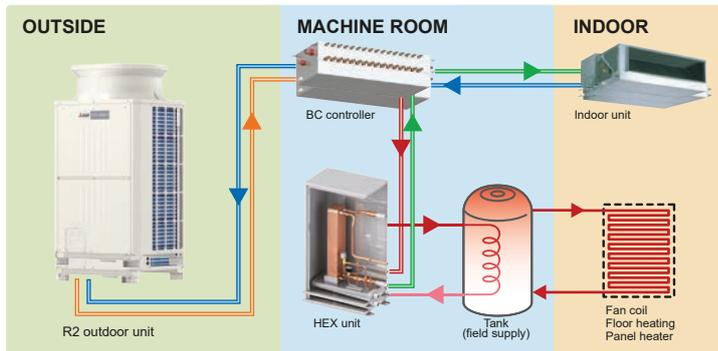
The HEX unit is connected to BC controller with refrigerant pipes, and to the water tank with water pipes. The HEX unit is not equipped with a compressor.
