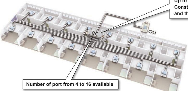
Up to 44HP can be connected to one main BC controller. Construction is easier as the number of piping connections and the suspension work can be reduced.
