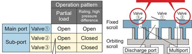
The sub-port is opened during partial load operation to discharge the over-compressed gas.
