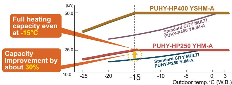
Using an industry first 'Flash-injection Circuit', the ZUBADAN System is able to provide FULL heating performance in ambient temperatures as low as -15°C.
