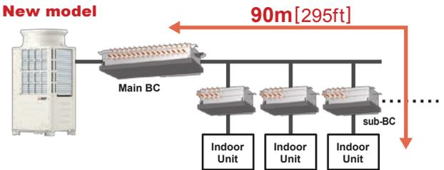
The piping length from the main BC controller to indoor units has been increased from 60m[196ft] to 90m[295ft], providing greater flexibility in piping design.
