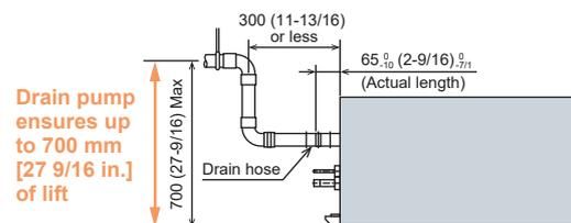
\*Comparison with drain pump PAC-KE04DM-F
