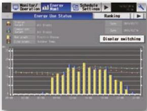
Energy consumption of applicable area is displayed by the month, day, and hour. Energy consumption of two different units, groups and blocks can be compared. Fan operation time as well as energy consumption can be displayed.
