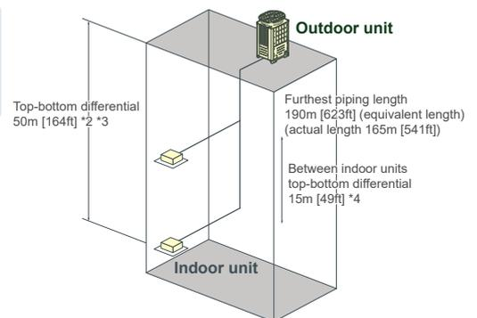
\*1 90m [295ft] is available. When the piping length exceeds 40m [131ft], use one size larger liquid pipe starting with the section of piping where 40m [131ft] is exceeded and all piping after that point.
