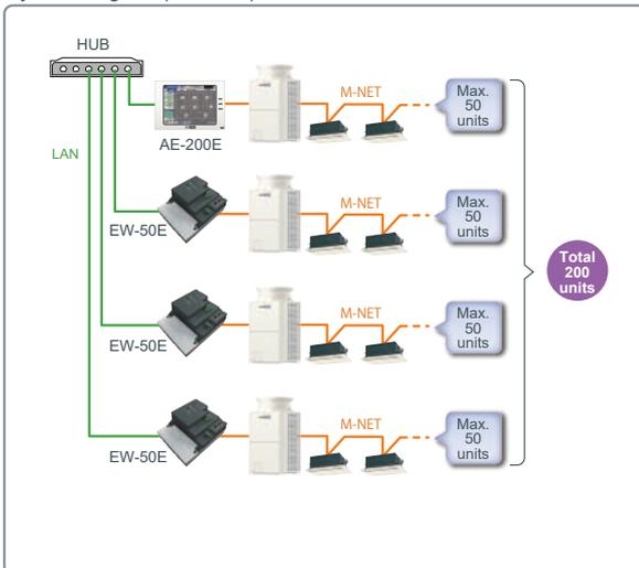
\* When M-NET of AE-200E is not used, a maximum of four EW-50E units can be connected.
