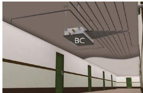
**(2) The line-branching method with a main BC controller and sub-BC controllers** New
