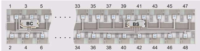
Branch piping from sub-BC controller is long
