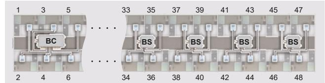
The sub-BC controller can be installed near the indoor units, so the branch piping can be greatly reduced. This also reduces the length of system piping, enabling using less refrigerant design.
