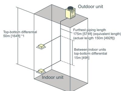
\*1 When the outdoor unit is installed below the indoor unit, top-bottom differential is 40m [131 ft].
