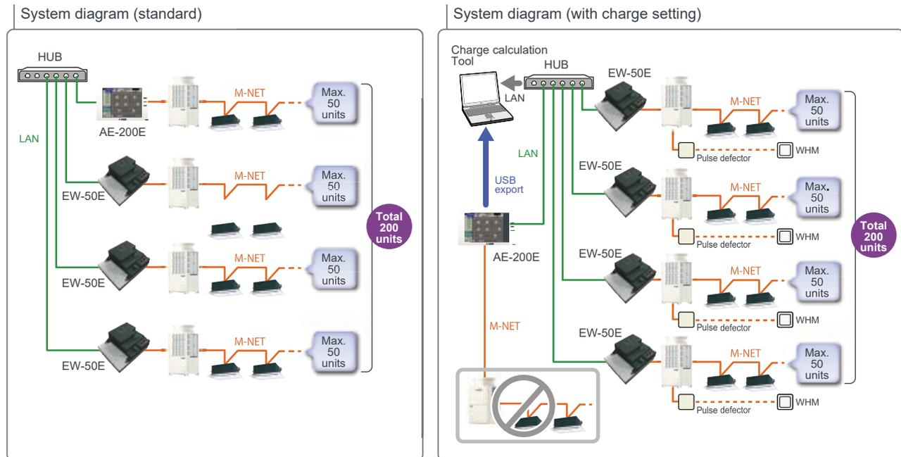
\* When M-NET of AE-200E is not used, a maximum of four EW-50E units can be connected.
