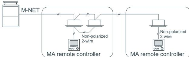
\*When a PAR-31MAAE is connected to a group, no other MA remote controllers can be connected to the same group.
