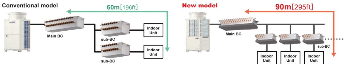
The piping length from the main BC controller to indoor units has been increased from 60m[196ft] to 90m[295ft], providing greater flexibility in piping design.
