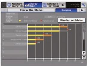
Energy consumptions of air-conditioning equipment are ranked and displayed by individual air-conditioning equipment and by area, thus visualising high-load components. Also, comparison of energy consumption with target electric energy is possible.
