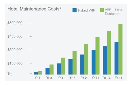
Throughout a system's lifetime, annual testing and the recalibration of leak detection sensors adds significant cost to a VRF system. Using Hybrid VRF instead, removes this need and could provide as much as 30% in maintenance savings over 15 years.
