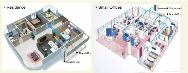
Consolidating heat sources for room air conditioners, which require a 1:1 connection between the outdoor unit and indoor unit, and reducing installation space is possible.
