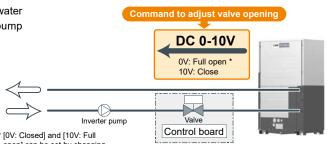
\* [0V: Closed] and [10V: Full open] can be set by changing the dip switch setting.
