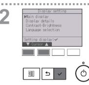
Move the cursor to "Main display" with the F1 or F2 button, and press the SELECT button.
