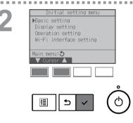
Move the cursor to "Basic setting" with the F1 or F2 button, and press the <u>SELECT</u> button.
