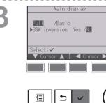
Select "B&W inversion" with the F1 or F2 button, and select the display mode "Yes" or "No" with the F3 or F4 button, and press the SELECT button. (The factory setting is "No.")
