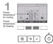
The current preset temperatures will appear. Press the  $\boxed{F2}$  or  $\boxed{F3}$  button to display the Settings
