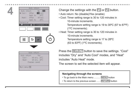
Timer or preset temperature settings will not be effective when the temperature range is restricted and when the system is centrally controlled (when the temperature range setting from local controller is prohibited). When the system is centrally controlled (when timer operation from local remote controller is prohibited), only the timer setting will be ineffective.
