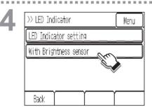
To select the brightness level of the LED indicator to be used when the brightness sensor detects "Light" or "Dark," touch the **[With Brightness sensor]** in the list.
