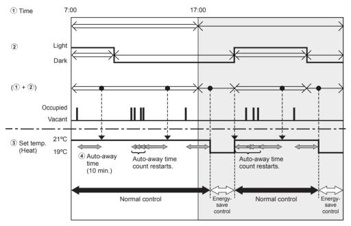
Period during which energy-save control can not be performed even when vacancy is detected
