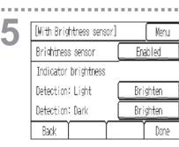
To use the brightness sensor for switching the brightness of the LED indicator, touch the **[Disabled]** button to change it to **[Enabled]**.
