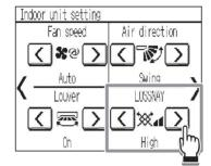
Touch  $\bigwedge$  or  $\searrow$  to go through the fan speeds of the LOSSNAY unit in the following order.
