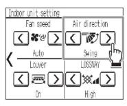
Touch  $\bigwedge$  or  $\bigwedge$  to go through the airflow directions in the following order. Select the desired setting.
