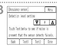
Set the detection sensitivity level with the 🔽 🛕 buttons.
