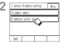
To set the threshold value of the brightness sensor, touch [Brightness sensor] in the list.
