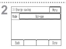
Touch the **[Mode]** button to select one of the following energy-save control modes that reduces energy-consumption during vacancy. The default setting is "Non-use."
