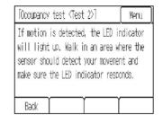
To start Test 2, touch **[Test 2]**. When movements are detected, the LED indicator will light up in blue. Walk away from the remote controller, and walk around in areas where you want the sensor to detect motions to see if it will respond correctly. If the sensor does not respond, raise the detection sensitivity level and try again.
