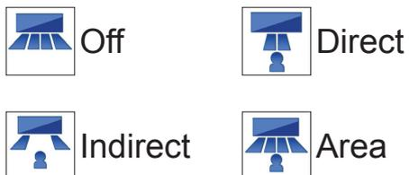
Note: When “Indirect,” “Direct,” or “Area” is selected, the vane angle and louver angle settings become “Auto.”
