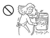
Washing the dehumidifier with water can result in electric shock and/or fire. In case of continuous drainage, protect the hose from falling below freezing point. (Refer to Page 17)
