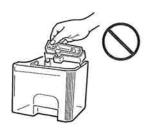
If it is removed, the float cannot detect the level of water filled to the brim, permitting water in the drain tank to leak down to the floor in the room, wetting household effects, etc., and can result in electric shock and electric leakage.
