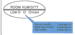
A temperature/humidity sensor is incorporated into this dehumidifier. When in Automatic Dehumidifying mode, dehumidification is performed according to the temperature and humidity in the room due to the function of the temperature/humidity sensor. At this time the LOW-HIGH humidity lamps will light depending upon the measured humidity.
