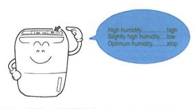
Dehumidification is performed according to the temperature and humidity in the room due to the function of the temperature/humidity sensor.
