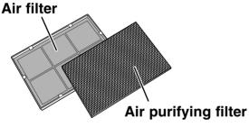
The air purifying filter cannot be washed in water
