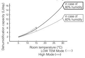
The dehumidification values shown on the graph were measured at constant temperature and humidity and do not reflect actual usage conditions.
