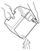
Empty the water tank and wipe away any remaining drops of water.
