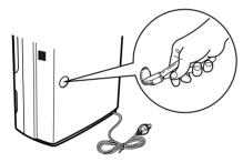
Use cutters to cut the three fixing ribs of the continuous drainage port on the back of the main unit, then remove it carefully making sure that it does not fall inside the unit.
