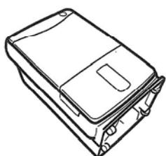
Inclining the unit may cause water in the tank leak into the unit **resulting in malfunction**. Should you incline the unit accidentally, contact your nearest dealer in order to discuss the matter.
