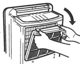
To remove press downwards the tabs on the air filter.
