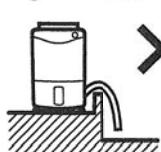
If any point of the hose is bent up, the unit's tank full detector will activate, and subsequently stop the unit making the continuous drainage operation impossible. It may also cause water leakage and/or electric shock.
