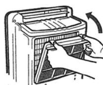
Insert the lower tabs into the main unit, then press the air filter until the tabs click into place.
