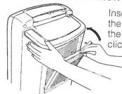
Insert the lower tabs into the main unit, then press the air filter until the tabs click into place.
