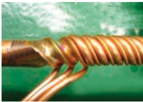
Twisted water pipe with the refrigerant pipe spiralled around it
