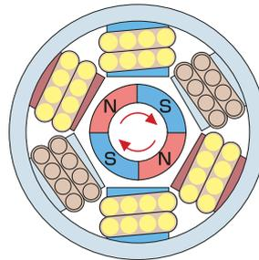
Brushless DC Motor with contact-free rotor eliminates wear and tear.
