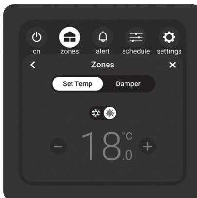
When the operation mode is Auto, the zone set temperature for cooling and heating can be set.
