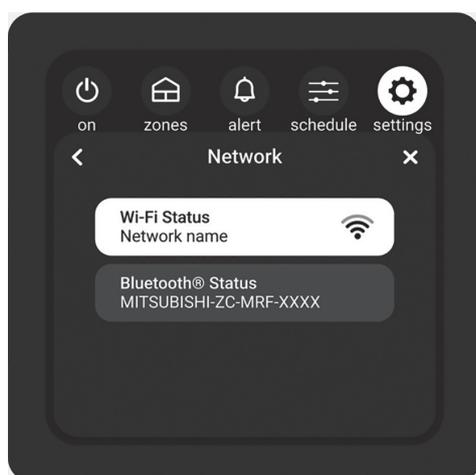
This controller connects to Wi-Fi for over the air updates for its firmware. In order to connect to Wi-Fi, you will be required to scan the code and download the Wi-Fi Control app. Connecting the controller to Wi-Fi is recommended for important updates for security, bug fixes, and other improvements.
