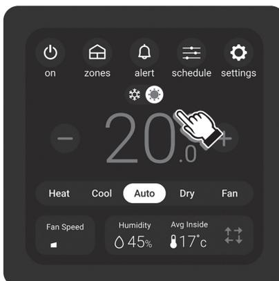
When the operation mode is AUTO, the set temperature for cooling and heating can be set.
