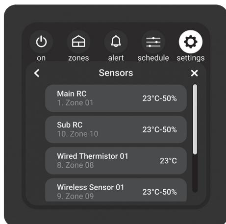
The sensor information in the system is displayed. If the sensor is selected as the representative sensor for a zone, the zone information is displayed.
