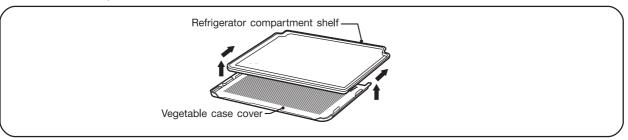
Insert the attached Vegetable case cover and compartment shelf into the rails (both left and right) upon the vegetable case.
