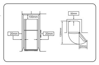
• Choose a location which is not exposed to sunlight, is relatively free from dust, heat and humidity, and offers good ventilation in order to guarantee that heat radiation will not be impaired.
