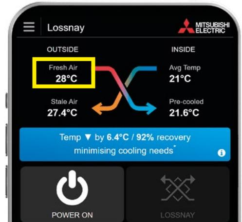
The outside air is drawn into and filtered through the Lossnay Core, where it crosses over the outgoing air-conditioned indoor air, which is showing as 21°C in this example.
