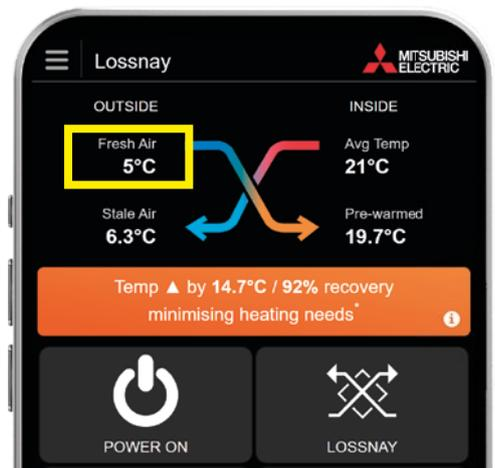
The cold incoming air is then increased by  $14.7^{\circ}\text{C}$  as it passes through the Lossnay Core.
