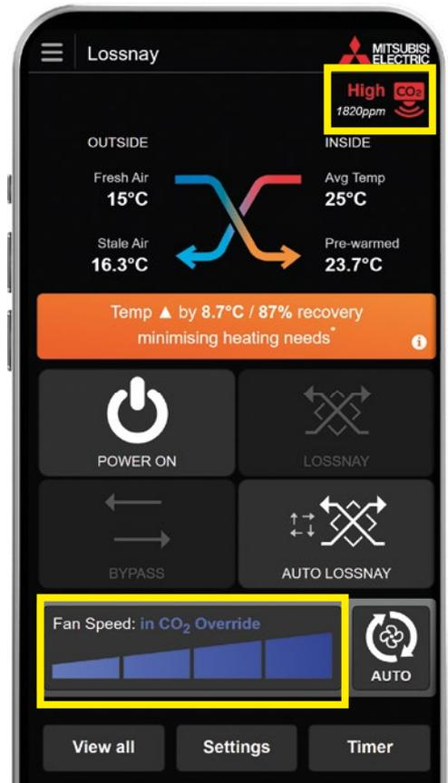
The system will continuously adjust the maximum volume of fresh air changes until optimum CO<sub>2</sub> levels are reached.
