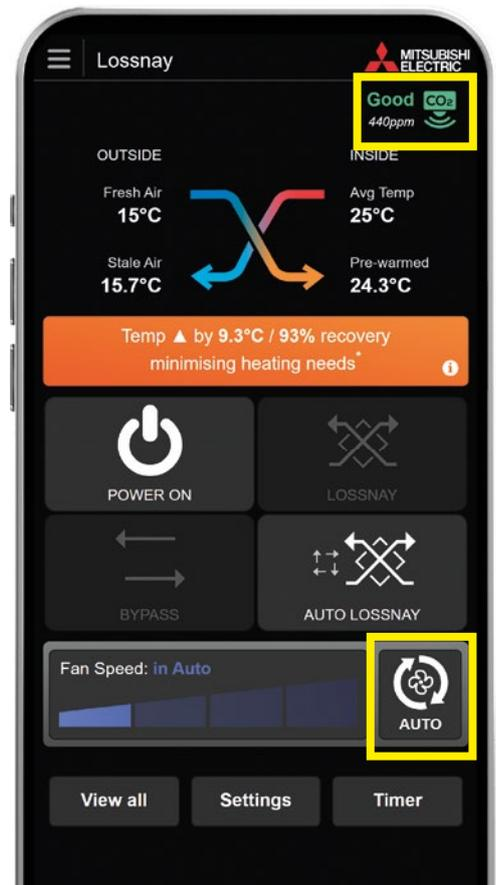
The highest Fan Speed level will activate when moderate or high levels of CO<sub>2</sub> are detected.
