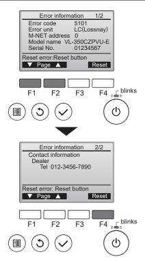
Error code, error unit, unit model name, and serial number will appear.
