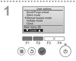
Setting method of the Manual bypass mode.
