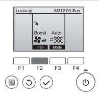
The Boost/Purge preset is the function that automatically sets the time to return to the [Base notch].
